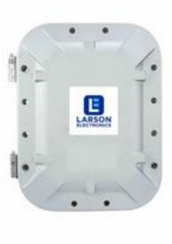
The Larson Electronics EPPB-TWI-MOD7 Explosion Proof Power Distribution Box is designed for safe disconnection of power in combustible work sites. Equipped with a 3-pole disconnect/isolator switch, the unit is rated 400V AC three phase 50 Hz (40 amps max). The IP66-rated enclosure is constructed of copper-free aluminum with stainless steel hardware (SS 304/316).
