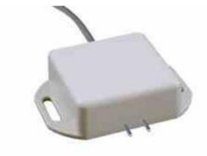
The EXP-EL-SR-IS-WS-FM from Larson Electronics is an Intrinsically Safe Floor Water Sensor capable of detecting water and conductive liquids in combustible environments. This unit does not consume electricity and comes with a normally open circuit configuration. Constructed of plastic with stainless steel conductivity electrodes, the immersion-type sensor offers instant response during use.
