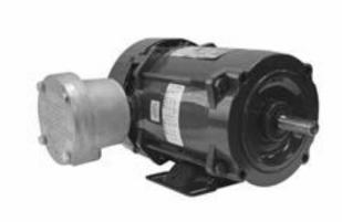
The Larson Electronics EXP-MTR-1P-230-1.5HP-1.8K-56H Explosion Proof Motor is recommended for use in Class I, Divisions 1 & 2 Groups C, D and Class II, Divisions 1 & 2 Groups E, F, G rated work sites. The 1.5 HP unit is compatible with 230V AC single phase 60 Hz and offers 7.8 FLA. This Class F insulation rated explosion proof motor features a NEMA 56H motor frame and can be installed with industrial systems via an integrated mounting foot.
