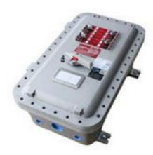
The EPPH-3P-208.120-225AMB-2X100A-4X20A is a lighting panelboard that is Class I Divisions 1 & 2 and Class II Divisions 1 & 2 explosion proof. This 225-amp main lug only panelboard is setup for 208Y/120 input voltage, has a 3-pole 4-wire configuration, and features two 100-amp breakers and four 20-amp breakers. The EPPH-3P-208.120-225AMB-2X100A-4X20A is constructed from copper-free aluminum.
