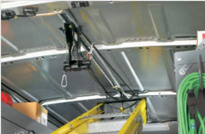
2 Slide the ladder forward along the rail.
