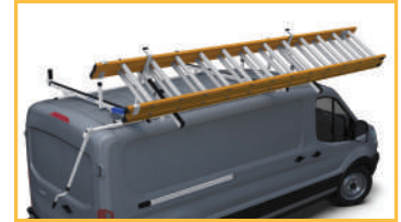
As handle is turned, the hydraulic assist begins to pivot ladder down
