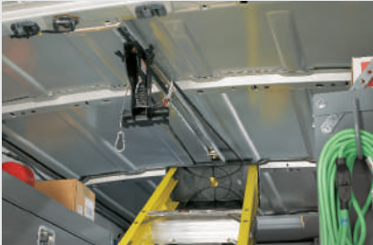
1 Hook the ladder onto the receiving pin.
