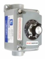
EXP-PTM.2K-2W Explosion Proof Potentiometer Listing: United States & Canada Unit Type: Explosion Proof Rotary Potentiometer Dimensions: 5.88" L x 3" W x 2.25" D Voltage: 30V DC Watts: 1 Configuration: Front Mounted Rotary Switch, 3 Wire pot Resistance: 200K ohm Resistance Unit Materials: Copper-free Cast Aluminum
