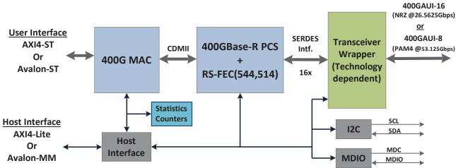
The 400Gbps Ethernet IP solution offers a fully integrated IEEE802.3bs compliant solution for use in core networks, Ethernet switching and network interface card (NIC) applications. The Ethernet cores implement an efficient architecture to achieve best in class resource utilization and performance numbers for targeting the complete 400Gbps Ethernet solution to ASICs as well as FPGAs.
