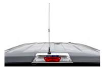
VMP-AM-GMC-SRA-2005-1500-LED Aluminum Plate For Mounting Permanent Mount Antennas
