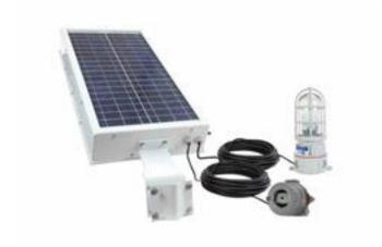
The Larson Electronics AVL-NVG-SOL-L810-LED-V1-30C Solar LED Strobe Light is an FAA AC 150/5345-43 Compliant unit with applications in aviation and harsh environments. This lighting system contains an infrared LED strobe light, powered by a 30-watt solar panel with a 40aH lithium-ion battery pack. A remote-mounted day/night sensor automates activation and deactivation during use.
