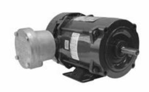
The Larson Electronics EXP-MTR-1P-115.230-2HP-3.6K-56HC Explosion Proof Motor is recommended for use in Class I, Divisions 1 & 2 Groups C, D and Class II, Divisions 1 & 2 Groups E, F, G rated work sites. The 2 HP unit is compatible with 115/230V AC single phase 60 Hz and offers 9.8 FLA. This Class F insulation rated explosion proof motor features a NEMA 56H motor frame and can be installed with industrial systems via an integrated mounting foot and C-face flange.
