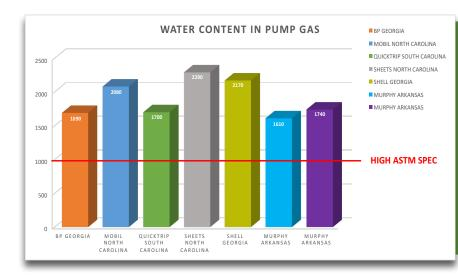
Modern gasoline is constantly changing, but not in a positive way as it relates to small engines. Ethanol content is rising. Fuel has inherent contamination, including water bonded to ethanol. The water problem becomes worse over time with condensation and water encroachment. WATER is the greatest enemy to your fuel system and engine. Ethanol attracts water and at some point this corrosive mixture phase separates to the bottom of your tank.
