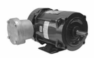
The Larson Electronics EXP-MTR-3P-230-0.75HP-1.8K-56C Explosion Proof Motor is recommended for use in Class I, Division 1 Groups C, D and Class II, Division 1 Groups E, F, G rated work sites. The 0.75 HP unit is compatible with three-phase 460V AC, 50/60 Hz and offers 1.4 FLA @ high. This Class F insulation rated explosion proof motor features a NEMA 56 motor and can be installed with industrial systems via an integrated mounting foot and C-face flange.
