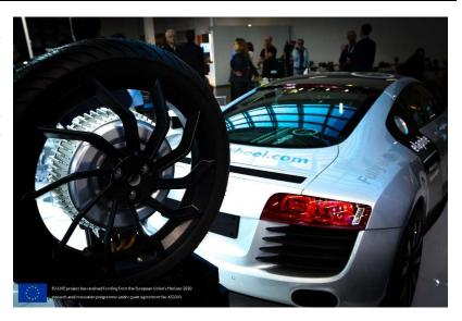
necessary), delivering upwards of 25 kW of power per wheel. The motors are designed to fit into the rear wheels of L-class vehicles. Directly-driven wheels vastly simplify the use tilting mechanisms, as the vehicle does not require any mechanical transmission.
