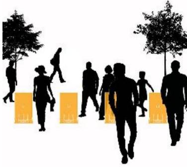
Portable barriers protect areas from vehicle entry while still allowing for unimpeded pedestrian flow.
