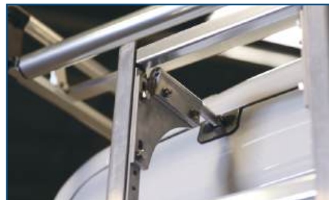
Padded top and bottom clamps attach to door edges without drilling
