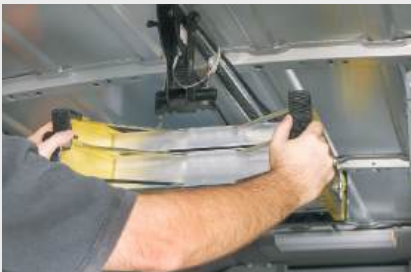
3 Raise the foot of the ladder to secure it to the catch bracket.
