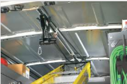
2 Slide the ladder forward along the rail.
