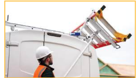
As handle is turned, the hydraulic assist begins to pivot ladder down
