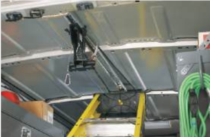
1 Hook the ladder onto the receiving pin.
