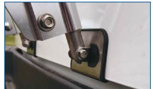
Padded top and bottom clamps attach to door edges without drilling
