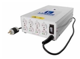
The Larson Electronics MT-MEX-ISX-120V-1.2KVA-4X5.15R Medical Isolation Transformer facilitates effective current isolation and power distribution in hospitals and medical buildings. This system features a 1200VA toroidal isolation transformer and four, 15-amp 5-15R 125V duplex hospital grade outlets. Protected by an aluminum enclosure, operators may bring power into the unit via 10' of hospital-grade cord with a 5-15P NEMA-rated cord cap.
