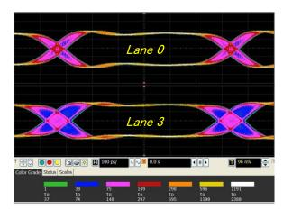
SV3C-DPTX provides individual jitter injection control for each lane
