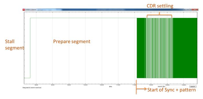
SV1C-MPHY Gear3 BER measurement in burst-mode
