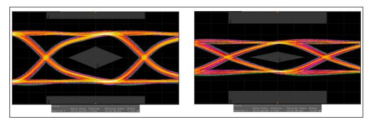
SV1C-MPHY Gear3 output eye diagram after long channel
