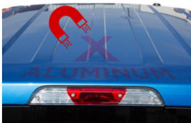
Aluminum Body is Not Magnetic
