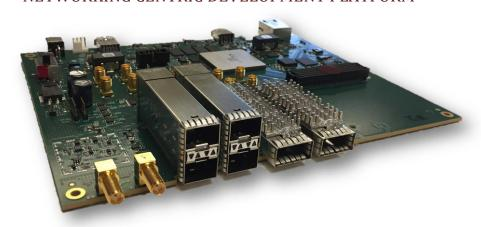
The Altera Arria SoC (10AS066-2E) based development platform is a network centric design with a single FMC mezzanine slot for application flexibility. All network and user interfaces are located on one edge and control / power on the opposite edge allowing for quick custom enclosure solutions. An integrated USB Byteblaster II is included for easy lab debugging.
