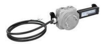
The Larson Electronics HAL-6-IPS-LED-1227 is a low profile hazardous location lighting solution approved for Class I Division 2 environments and UL 1598 compliant for use in wet locations. This powerful 6" long LED strip light produces 750 lumens, operates on 120/240V AC, and is suitable for a variety of applications.
