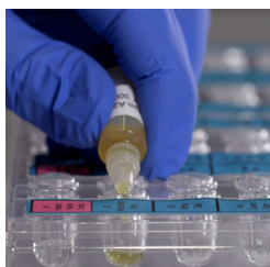
FILLING the dip wells
