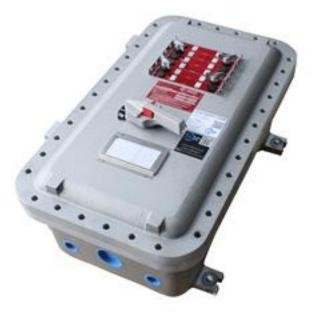
The EPPB-3P4W-208Y.120-100AMB-5X120-5X208 Explosion Proof Panelboard offers circuit management and protection in hazardous locations and indoor/outdoor work sites. The 100-amp rated main circuit breaker panel is compatible with 208Y/120 three phase and comes with five, 20-amp 208Y and five, 120V breakers. The 25-circuit panel is constructed of copper-free aluminum.
