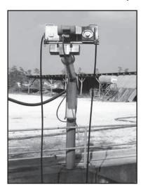
through scrapers and returns the clean tube to the water surface to gather more oil. The collector tube, which is sized to your application. snakes over and around floating debris to reach contaminant The flexible tube flops so that it breaks through crusted oil or grease and makes these contaminants adhere to the outer surface. The tube will extend as far as 16 feet from shoreline or pit edge when the 6-V is equipped with our balanced boom system.
