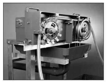
Moveover, Oil Skimmers can outfit the 6-V mechanism with heating elements to keep the oil moving in the coldest weather. For applications where there is exposure to high acidity or other harsh external environments, Oil Skimmers can treat all external metal parts with a special coating for added protection.
