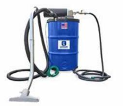
The Larson Electronics EPV-PN-55G-48CFM-1.5IN-15D is an Explosion Proof Vacuum for flammable environments and industrial applications. This 55-gallon unit features an anti-static hose, 18 gauge steel drum and a swivel caster base for seamless portability. The certified HEPA explosion proof vacuum is equipped with a 3/4" x 20' anti-static air line for power.
