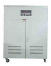
The Larson Electronics IND-SFC-3P-15KVA-380-50HZ-240-60HZ Solid-state Voltage Frequency Converter is designed for voltage and frequency rectification in industrial locations. The 15 KVA converter comes with an input voltage/frequency of three-phase 380V Delta, 50 Hz and an output voltage/frequency of three-phase 240V Delta, 60 Hz. This unit is mobile via four wheels at the bottom of the enclosure.
