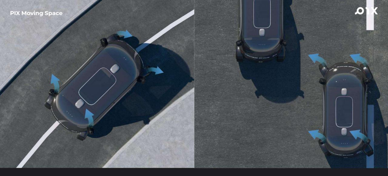
4-wheel differential steering to navigate through narrow roads
